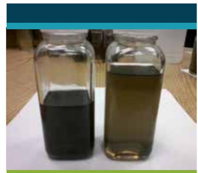
Photo of the dirt dispersing abilities of the LAC 945 (left) at 15% to the competitive fluid at 100%.
