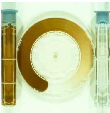
**Figure 10** - Illustration of a portable calorimetric test for the presence of nitrite corrosion inhibitor.
